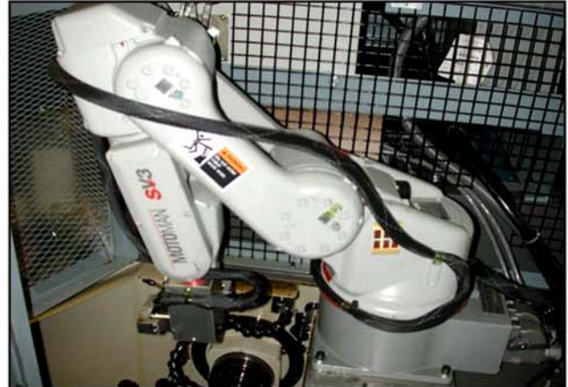
Motoman 6-axis Robots enables us to load parts with precision accuracy for 2nd operation machining.
