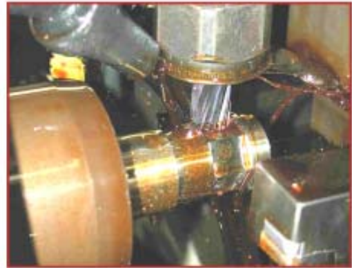
Overhead Vertical In Process Milling
